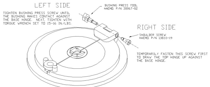
4. Using the 1/2" box wrench, fasten the left side of the cover hinge using the Bushing Press Tool, P/N 38067-02, and tighten until the bushing makes contact against the base hinge. (This tool will physically push the bushing into the cover hinge.) Next, tighten the Bushing Press Tool with a torque wrench set to 15/16 in./lb., until the click of the torque wrench is heard. This will ensure a firm press of the bushing against the base hinge. (See illustration below.)
