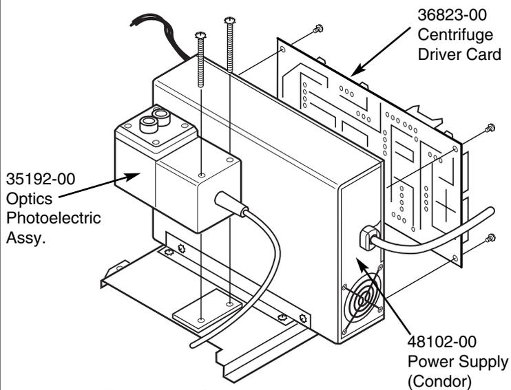
If replacing a Todd Power Supply with a Condor Power Supply, order P/N 48895-00 Condor Power Supply (Field Replacement).
