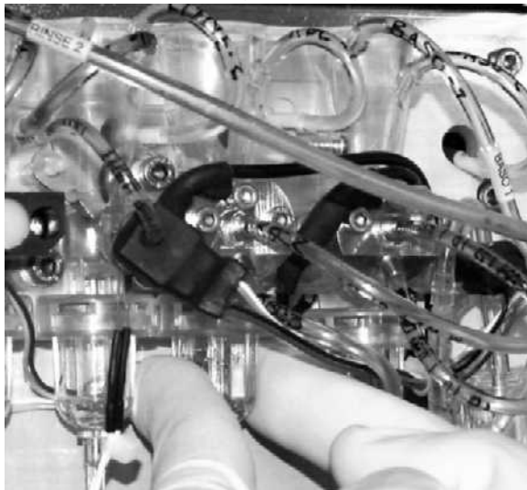
Figure 4.34-1 Removing a Draining Bath
