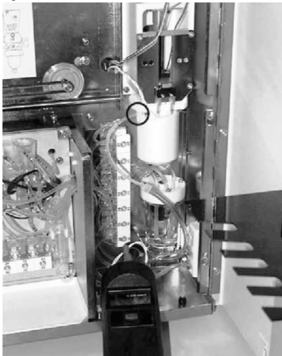
Figure 4.17-1 Attach the Vacuum Meter to the Waste Syringe
