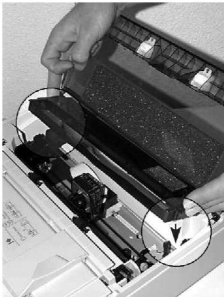
Figure 3.3-3 Insert the Ribbon Cartridge
