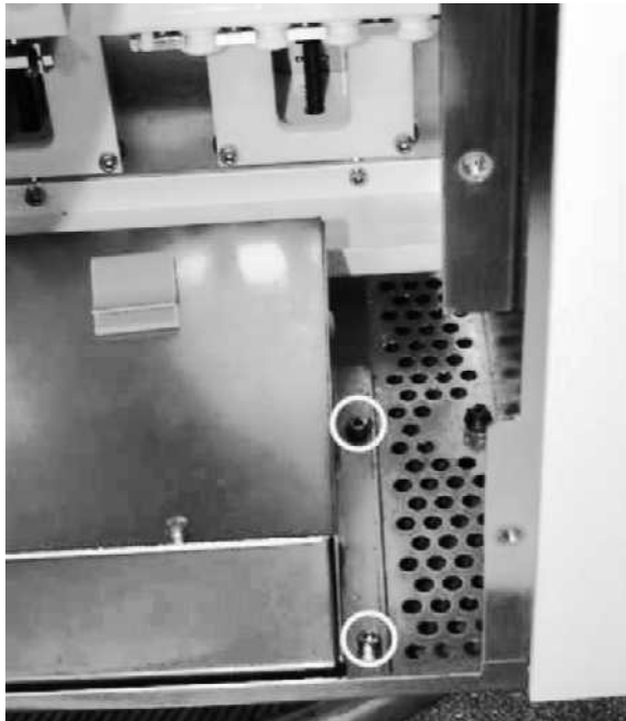
Figure 4.20-5 Screws Securing the Power Supply to the Instrument Frame
