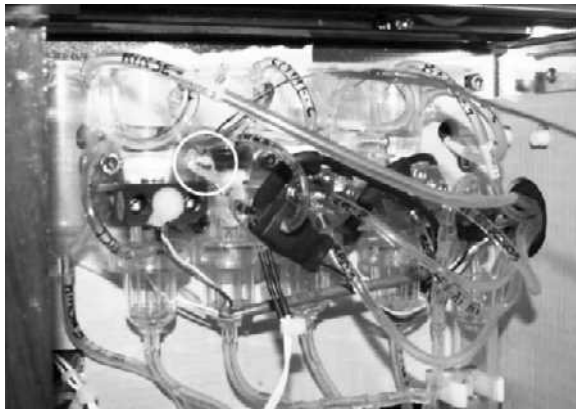
Figure 4.16-1 Temperature Sensor Location - View with the Right Side Door Open
