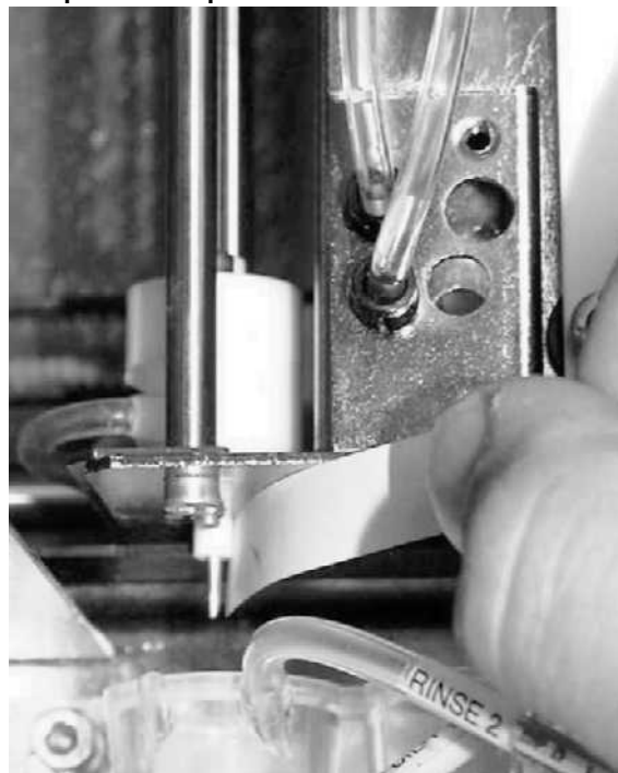
Figure 4.6-3 Measuring the Distance between the Sample Probe Tip and the Traverse
