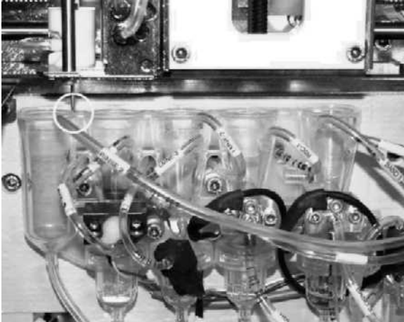
Figure 4.5-1 Sample Probe Position at the Rinse Bath
