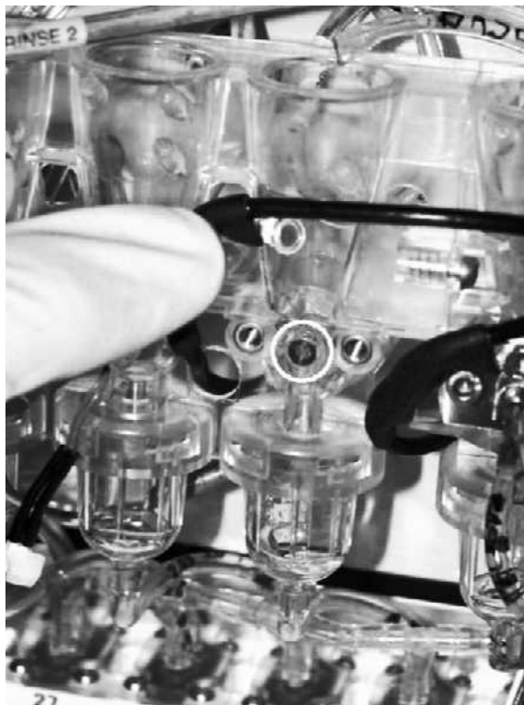
Figure 4.35-8 Location of the Aperture and Its Two O-Rings
