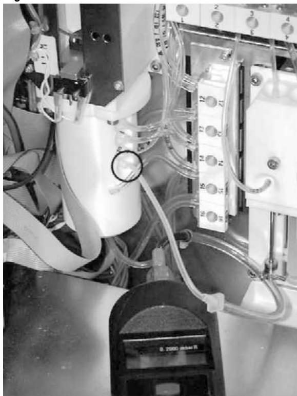
Figure 4.17-2 Attach the Vacuum Meter to the Count Syringe
