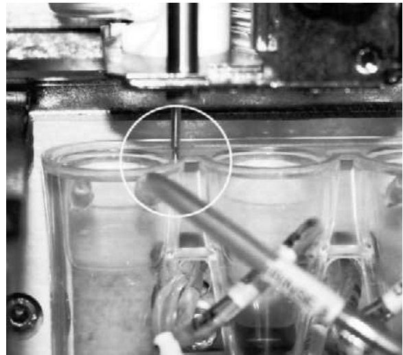
Figure 4.5-7 Close-up of Acceptable Probe Position
