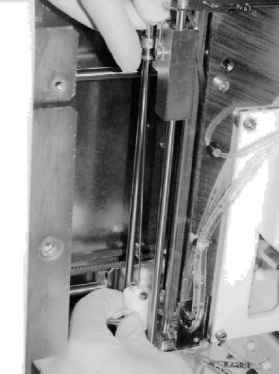
Figure 4.26-3 Remove Probe and Rinse Block Assembly
