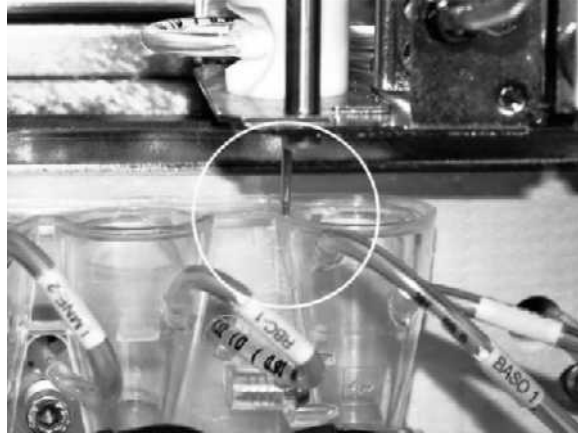
Figure 4.5-9 Close-up of Acceptable Probe Position
