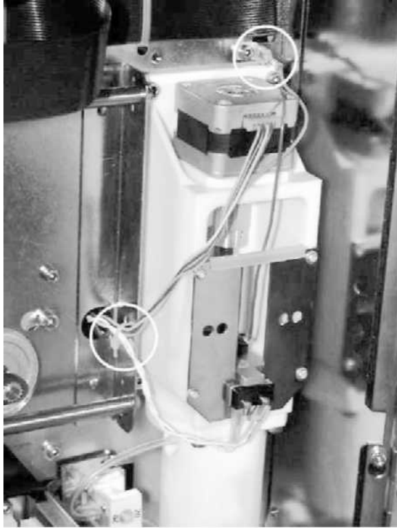
Figure 4.27-3 Waste Syringe - Tie Wrap and Ground Wire Location
