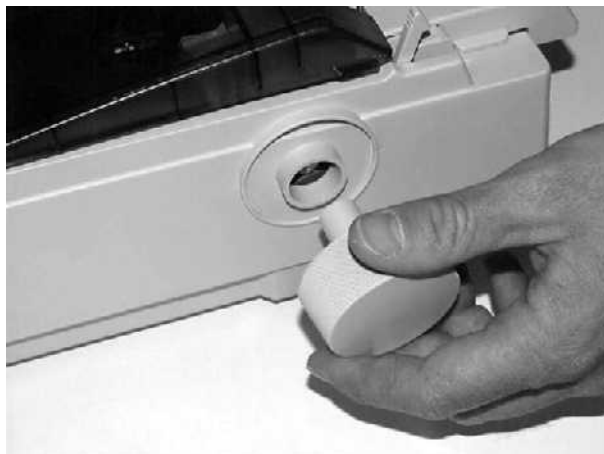
Figure 3.3-2 Paper-Feed Knob Installation
