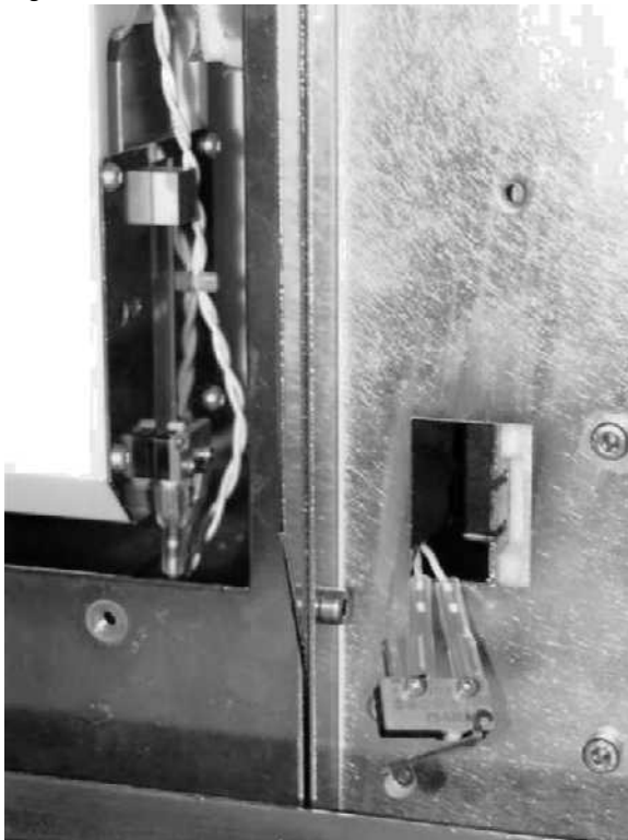
Figure 4.21-3 Disconnected Start Switch - Front View with Front Panel Removed
