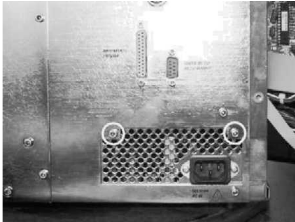
Figure 4.20-4 Location of Screws Securing the Power Supply to the Rear Panel
