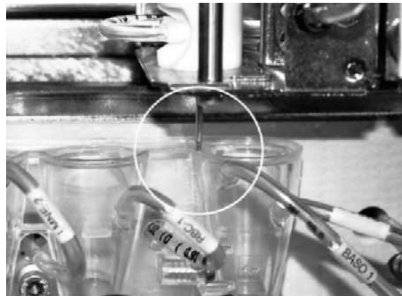
Figure 4.5-4 Close-up of Probe at the WBC/BASO Bath
