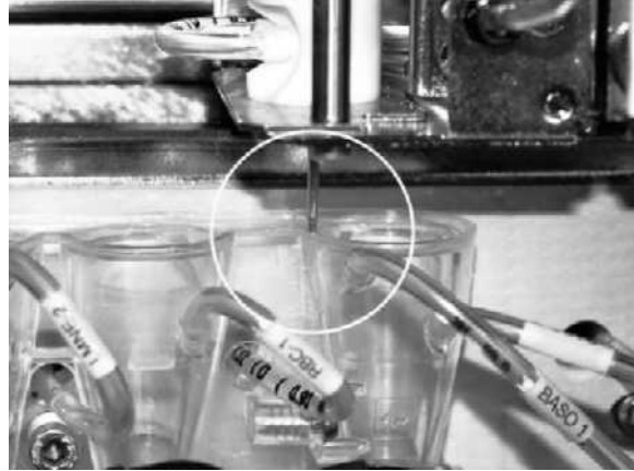
Figure 4.35-12 Close-up of Acceptable Probe Position
