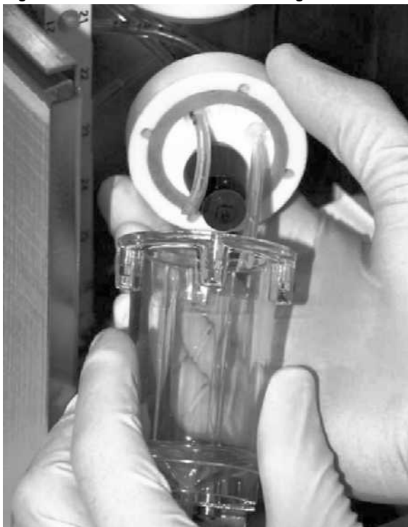
Figure 4.32-2 Diluent Reservoir O-ring and Washer Positioning
