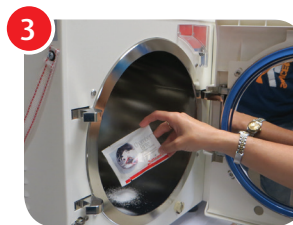
3 Open the door and spread the contents of a packet of Chamber Brite™ in a straight even line along the bottom of a cold chamber, from back to front.
