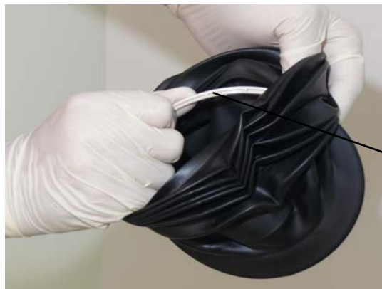
FIGURE 7-8 Removing the Bellows Adapter Ring
