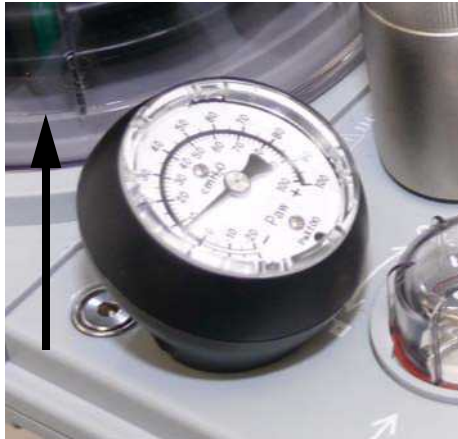
FIGURE 7-15 PAW Gauge Removal
