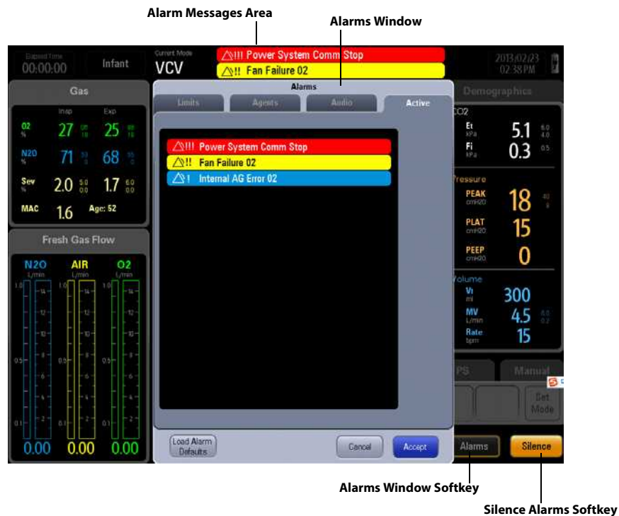
FIGURE 6-1 Alarms and messages on the main screen and in the Alarms window
