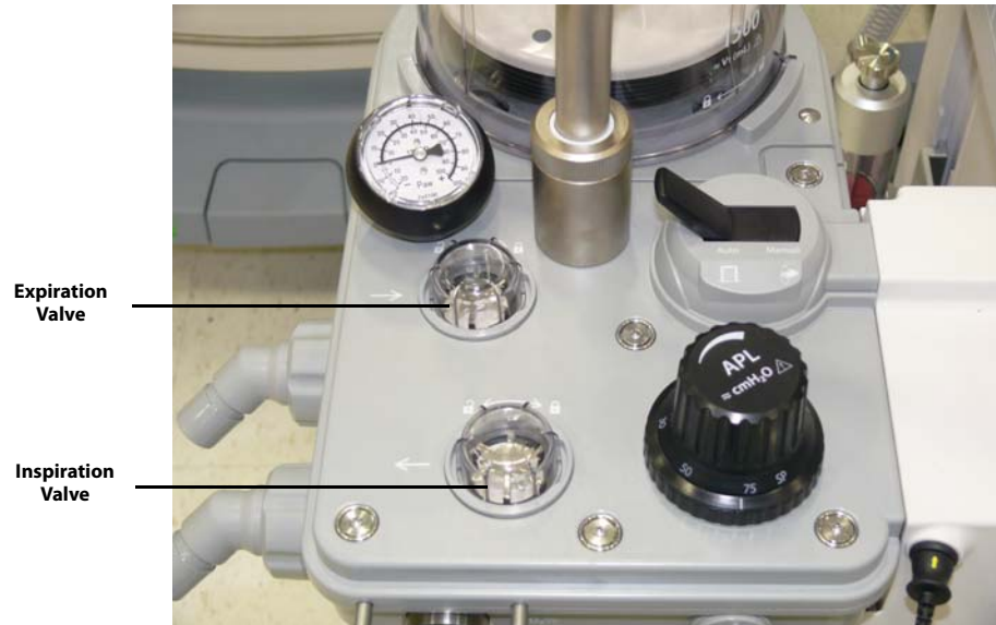
FIGURE 7-10 Location of Expiration and Inspiration Valves
