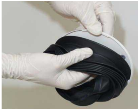
FIGURE 7-7 Detaching the Bellows Top Plate
