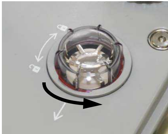
FIGURE 7-11 Valve Dome Removal
