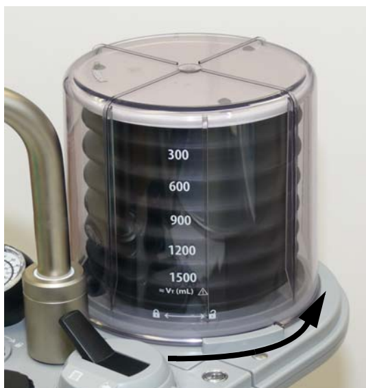
FIGURE 7-5 Removing the Bellows Dome
