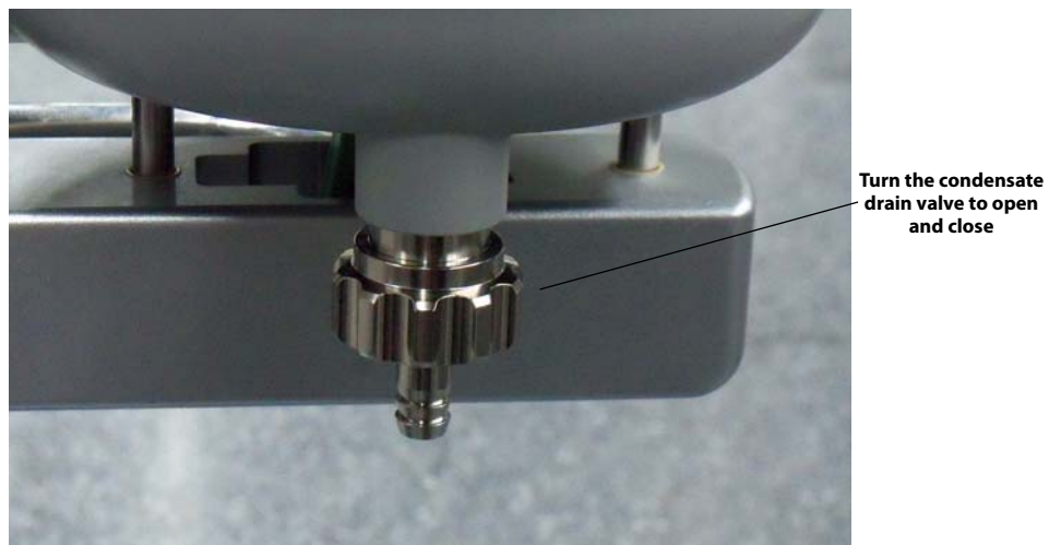
FIGURE 7-18 Condensate Drain Valve (Close Up View)
