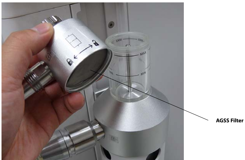
FIGURE 7-24 Removal of AGSS Top / AGSS Filter Inspection
