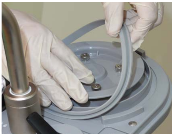
FIGURE 7-9 Removing the Bellows Dome O-ring
