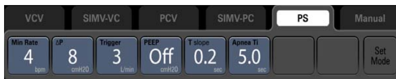
FIGURE 3-24 Ventilation Mode: PS
