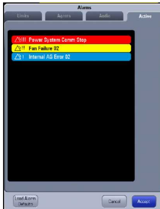
FIGURE 6-2 Active Alarms list in the Alarms window
