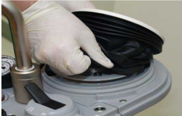
FIGURE 7-6 Detaching the Bellows
