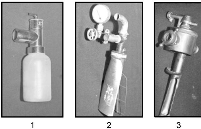
The most common vaporizers incorporated in the anaesthetic machines available in India were the Boyle's ether and trilene bottles. Many other vaporizers became popular before the tec series of vaporizers became standard. Though popular during the early 1970's they are still being used in many places.
