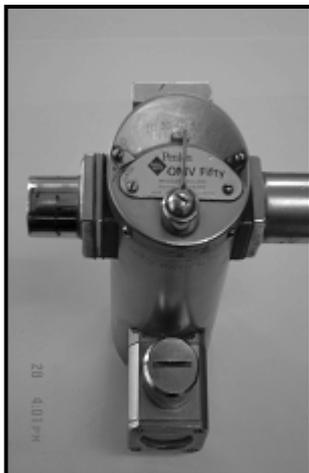
Manufactured by 'Cyprane' this was designed for halothane but has a dial for chloroform and trilene.
