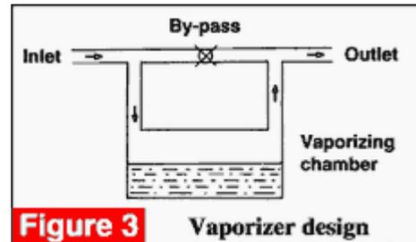
**Figure 3** Vaporizer design
