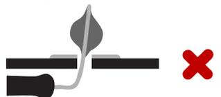
A spike of solder means that the joint has been overheated.
